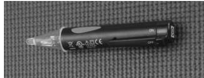
Figure 22 - Use a non-contact circuit tester to check for electrical power.
